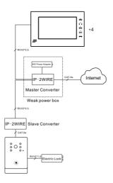
IP-2WIRE Converters are used to extend the Ethernet IP signals via 2Wire cable in the existing 2Wire network of building.
